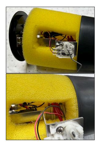
23. Install the fuel pump adapter plug/wires to the appropriate electrical stud in the billet top plate.
