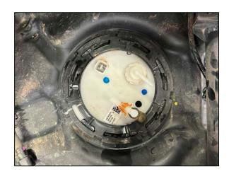
9. Apply a mark on the fuel tank and on the fuel tank locking ring at the point where the arrow is molded into the top of the gas tank. This will help when reassembling the fuel tank ring later on.
