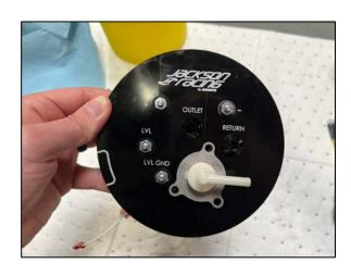
17. On the underside of the billet fuel pump top is a pipe plug next to the fuel pump exit hose. Remove that plug and install the Aeromotive 50psi fuel pressure set-valve. Wrap the threads with a small amount of Teflon tape prior to installing and tightening the fuel pressure set-valve. This may be preinstalled.
