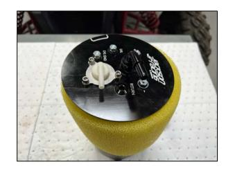
20. You will find two remaining threaded holes in the underside of the billet top. These holes are for the fuel level sender bracket. Install the pump down into the fuel cell foam. Carefully work the pump down into the foam while lining up the two threaded holes on the underside of the billet top with the cutout in the fuel cell foam that is exposed above the fuel bladder.
