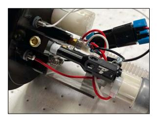
18. On the top of the Jackson Racing fuel pump you will see two holes. One marked OUTLET and one marked RETURN. Install the -6 ORB plug provided in your kit to the hole marked RETURN. Apply a small amount of lubricant to the O-ring prior to installation. Tighten the plug until the O-ring seats. If plug was pre-installed, double check if it is tight.
