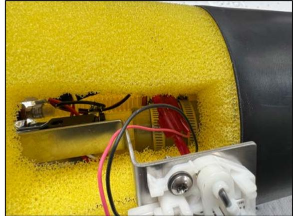
21. Install the fuel pump adapter plug/wires to the appropriate electrical stud in the billet top plate.
