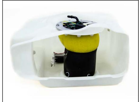
23. Reinstall the fuel pump locking ring and using the special tool turn the locking ring until the marks that you put on the locking ring align with the mark you put on the fuel tank. This is just as hard installing as it was getting off. Be prepared to push hard.
