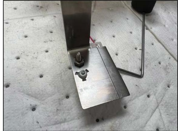
15. On the underside of the OEM plastic fuel assembly top plate you will need to lift up the small retaining clips to allow the “roll-over valve/vent assembly” to be pushed up and out of the top of the OEM plastic housing.
