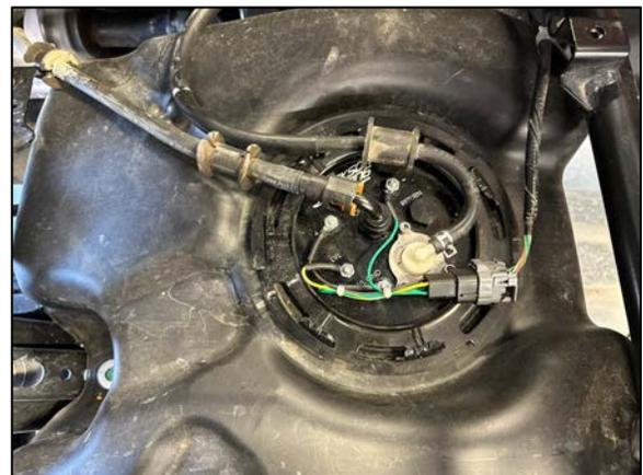
29. Plug the wiring adapter into the OEM wiring plug at this time.
