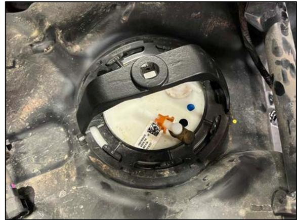
10. Drain as much fuel from the fuel pump bucket into the fuel tank before pulling the pump completely out of the tank. Cover the open fuel tank with a shop towel.
