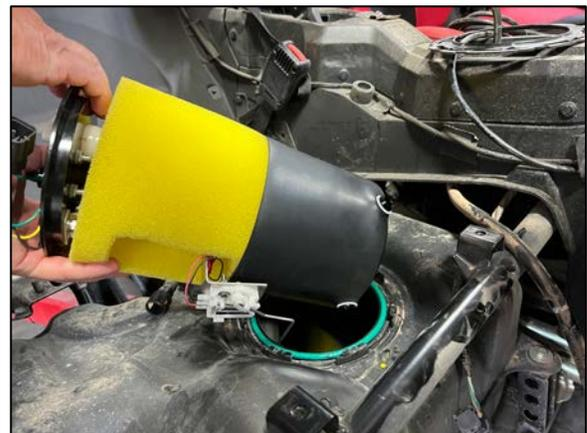
should be on the back side of the fuel tank with the float facing towards the center console.
