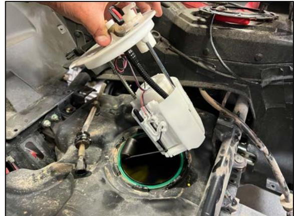
11. Cut the fuel level sending unit's red and black wire approximately 5” from the sending unit.
