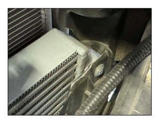
The horizontal air director needs a small trim to fit snug to the intercooler core. This is a great OEM airflow piece that we take advantage of with the stepped core. Do not skip installation!
