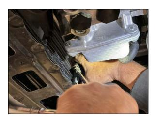
Refer to the photos for trimming of the vertical shrouds on the side and slowly trim the plastic until it fits snugly around the intercooler. Notice we used a Sharpie to mark an approximate edge and trimmed from there. You can clean the sharpie off with some contact cleaner when trimming is complete.
