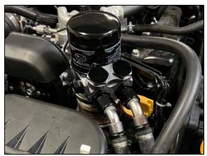
32. Reinstall your headlight assembly. Double check the oil hose routing. Make sure the hose is not rubbing on any sharp edges throughout the entire installation.
