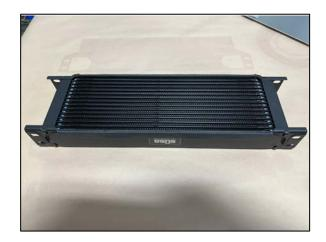
23. Install the Shroud Top and Bottom using two (2) M6x1.0x25mm bolts on top and four (4) M6x1.0x18mm bolts on the bottom. The top two are just temporary, as this whole assembly will be mounted to the bracket on the car later on.
