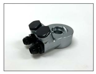
12. Install the Thermostatic Oil Cooler Adapter, with the -10AN fittings loosely installed, onto the previously installed adapter spacer. The O-ring side of the sandwich adapter should be placed against the smooth side of the aluminum adapter spacer.
