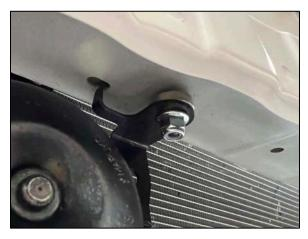
18. On the driver side of the front bumper support you will find an open mounting hole with no threads that is approximately 23" from the stud mounting location. Reach in through the opening in the front bumper support and install a M6x1.0x25mm flanged bolt (91100-06025) with a M6 fender washer down through this mounting hole.
