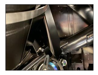
43. Install the new Jackson Racing Air Filter onto the "velocity stack" inlet connector. Secure with the hose clamp provided. Install the foam "large particle filter" over the air filter assembly. Apply a small amount of thread locking adhesive to the two 6mm studs found in the air filter hardware kit and install them into the threads in the "velocity stack". The air filter is ready to be installed in the air filter housing.
