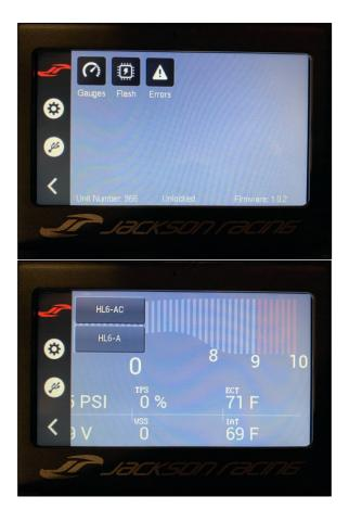
Let ECU Flash process go through. Again, do NOT turn off the vehicle. Do NOT have voltage fluctuate in any way during reflash procedure. If you forgot to turn your headlights off, that is okay. Do NOT turn them off while flashing.
