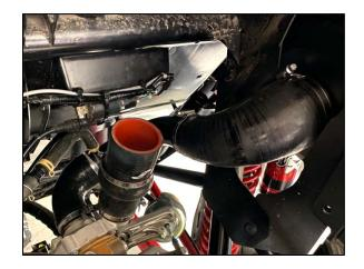
Straighten the bend in the hose and mark 3" up from the end of the hose and cut the angle off of the hose at that point. Straighten the OEM air filter drain hose and make a mark at 5" up from where the short bend ends. This will be the end that doesn't have the white drain plug fitting in the end of the hose. Cut the hose at that point. Join the two cut hoses together with the .5" hose connector supplied with your kit. DO NOT reuse the white Honda connecter, it is not a through connector.
