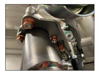
35. Connect the AN10 x 90° side of the drain hose to the turbo. If the 90° fitting isn't pointing directly at the drain fitting on the turbo you can rotate the fitting in the hose. Grasp the fitting and the hose and twist until the desired angle is achieved.
