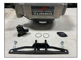
54. With the TURBO badge facing towards you, install the Jackson Racing/Turbosmart recirculation valve on the left side of the intercooler using one of the O-rings and two M8x1.25x25mm Allen Head Cap Screws (AHCS) provided. Mount it so that the horizontal 1" spigot faces towards the intercooler core and not away from the core.
