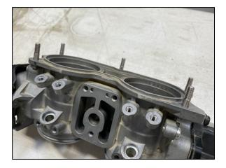
23. Locate the Intake Air Temperature (IAT) sensor from the stock air filter assembly. Install the new <sup>3</sup>⁄<sub>4</sub>" outside diameter O-ring supplied. This O-ring seals the sensor to the new cast intake manifold. Install the sensor with O-ring and cover plate onto the intake manifold with two 4mm screws. Apply a small amount of thread locking adhesive to the two screws prior to installing them.
