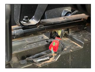
62. Unbox your Jackson Racing ECU Flash Tool and connect the included ECU harness to the rear of the Flash Tool. Now plug the male connector into the Red female data connector. (4 Pin model shown to the right)
