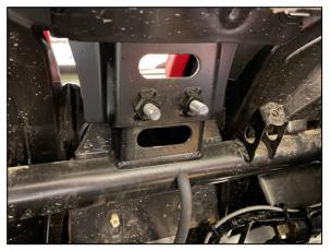
56. Locate the Upper Intercooler Chassis mounting bracket. This bracket will have two mounting holes in it and one mounting rod for the rubber mounting grommet to hang from. Make note of the bracket orientation, as installing upside down will hinder intercooler installation.
