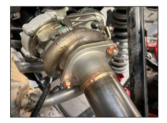
34. Now that the muffler and turbo-exit studs are tight it's time to torque the turbocharger in place. This process is always easier with two people. Using one person to tighten the bolts from above while another person holds the nuts from below torque all three mounting bolts to an initial torque setting of 20 ft-lbs. Now increase the torque on all bolts to 30 ft-lbs.
