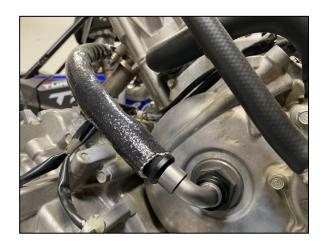
27. Route the turbo oil drain hose from the front of the alternator cover towards the future turbo location. It will be routed below the horizontal radiator hose and above the main horizontally mounted wiring harness. Additionally, it will also be routed between the EVAP hose (where applicable), the vertical differential vent hose and the plastic wall between the driver compartment and the engine.
