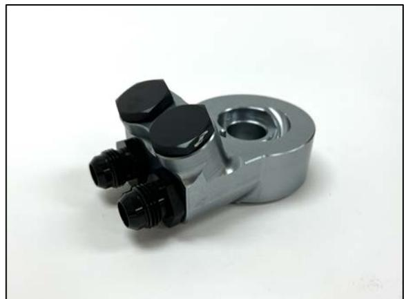
26. Install the Oil Cooler Adapter, with the -10AN fittings loosely installed, onto the previously installed adapter spacer. The O-ring side of the sandwich adapter should be placed against the smooth side of the aluminum adapter spacer.
