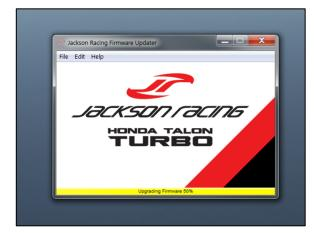
5. Once complete, you will get a window confirming your firmware is up to date. Select OK. You will see the green bar at the bottom of the application window. The green bar will then turn yellow and the updater will begin installing the most current calibration files to your Flash Tool. "Uploading a file" will appear on the Flash Tool screen. This can take up to 5 minutes. Once complete, the bar will turn back green.
